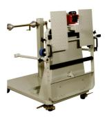
To facilitate the loading of stock drums the optional payout module is fitted to the rear of the machine, thus making the machine an all in one winder and payout.
